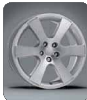
Alloy wheel - 19" 6 spoke, excl. wheel nuts. Diamond cut surface. Recommended tyre size 245/45R19. MME31522
