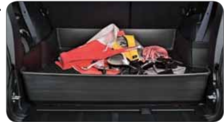
◀ Trunk tray Flexible shell with low edges (5 cm). For vehicles without Rockford Fosgate MZ313912 For vehicles with Rockford Fosgate MZ314112
