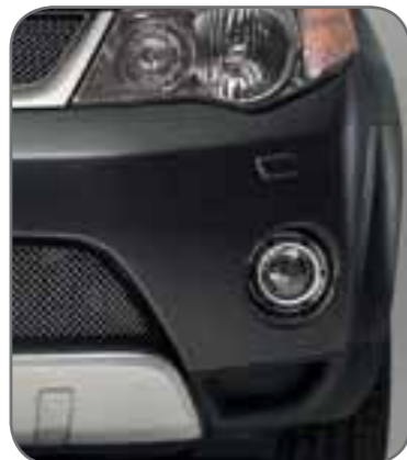
◀ Fog lamp kit ▶ Clear lens, 90 mm, silver bezel. For Invite models only. MZ380460EX
