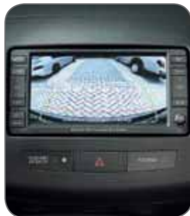
◀ Rear view camera kit ▶ Only in combination with MMCS unit. Camera installed above the licence plate. MME31844
