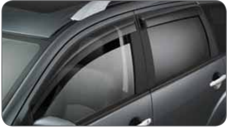
▶ Side window deflectors For front and rear doors. MZ380358EX
